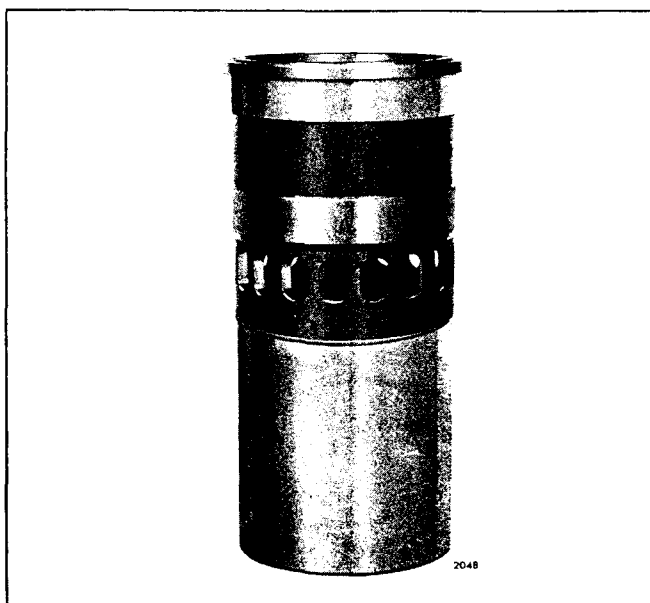
Fig. 1 - Cylinder Liner
