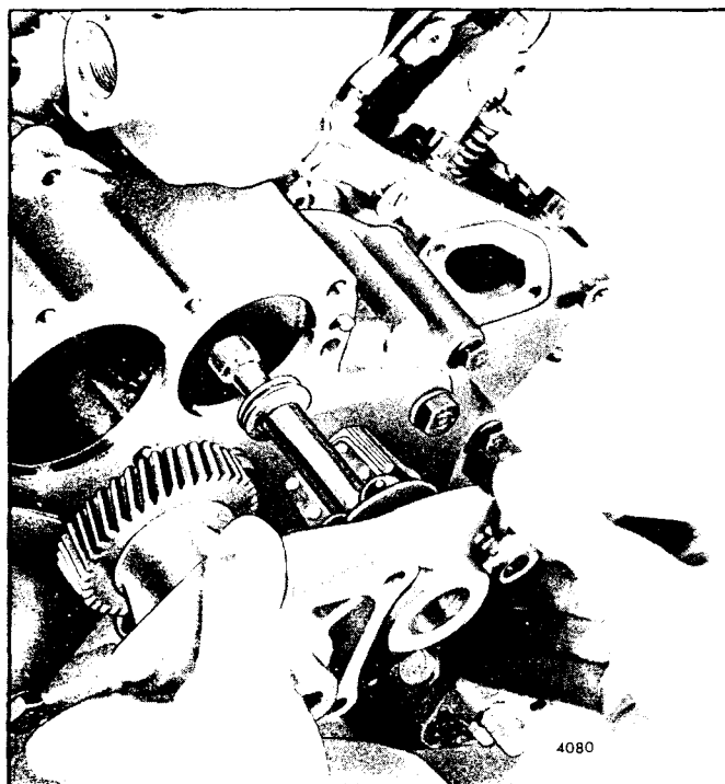
Fig. 3 - Removing or Installing Blower Drive Support
