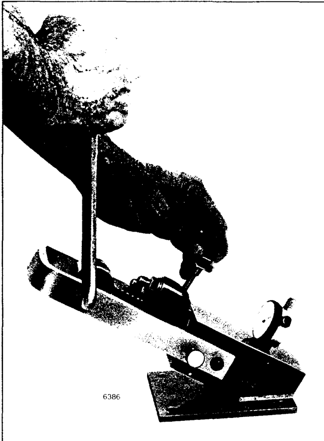
Fig. 35 – Checking Rack for Freeness in Tester J 29584
